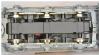
The improved bottom gear cover is designed with longer pegs to better capture the truck sideframes solving the bearing cap problem.
