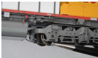
Positioning the bearing cap
