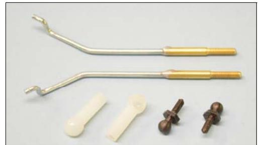
OUR 5250 LINKAGE KIT PROVIDES MORE PRECISE STEERING AND CAN BE ADJUSTED BY SNAPPING OFF THE BALL CUPS AND THREADING THEM FARTHER ON OR OFF THE THREADED ROD. THE WIRE LINK CAN BE RE-BENT TO SUIT MOST MOUNTINGS.
