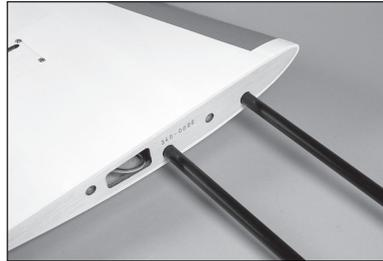
56. Use a hobby knife with a #11 blade to remove the covering for the two wing bolts and the opening for the servo leads on both sides of the fuselage.
