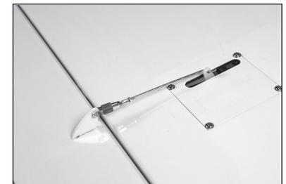
44. With the flap servo centered using the radio system, adjust the linkage to achieve the 1 inch (25mm) mid-flap throw.
