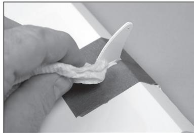
11. Before the epoxy fully cures, remove the tape from around the control horn. This will allow the epoxy to flow around the control horn, creating a small fillet between the control horn and surface for a finished look and secure bond. Allow the epoxy to fully cure before proceeding.
