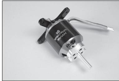
**113.** Use two M4 x 20 socket head cap screws, two M4 washers and two M4 lock nuts to temporarily attach the motor to the motor box plate
