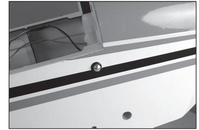
**161.** The vent line fitting is mounted on the underside of the fuselage. Attach the vent line to the fitting.
