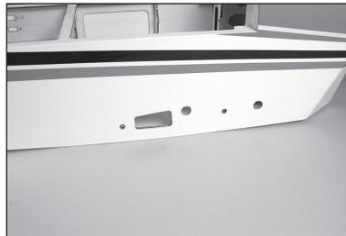
57. Slide the wing panel into position. Guide the flap and aileron leads into the fuselage.
