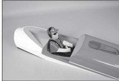
175. Use canopy glue to attach the canopy to the cockpit. Use low-tack tape to hold the canopy in position until the adhesive fully cures.
