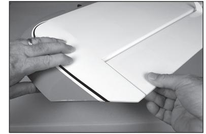
22. Break in the hinges by flexing the control surface through its range of motion in both directions.
