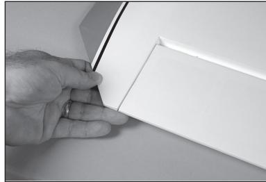
18. Check the gap between the aileron and flap.
