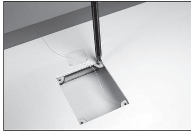
26. Apply 1–2 drops of thin CA in each hole to harden the surrounding wood. Allow the CA to fully cure before proceeding.
