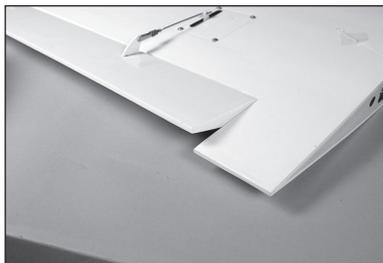
45. Move the control at the transmitter to the raised flap position. Adjust the throw percentage of throw at the radio to align the flap with the trailing edge of the wing at the root.
