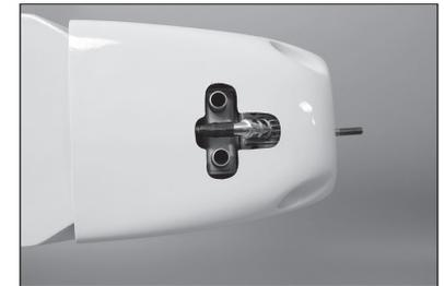
**165.** Fit the spinner cone to the spinner backplate to continue checking the cowl alignment. The cowl will sit slightly higher than the spinner, which is scale for this aircraft. There will be a 1/8 inch (3mm) gap between the spinner backplate and front of the cowl.
