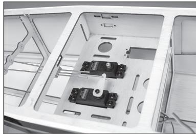
97. When attaching the linkage to the servo arm, use the hole that is 1 inch (25mm) from the center of the servo horn. This hole will need to be enlarged using a pin vise and 5/64-inch (2mm) drill bit.
