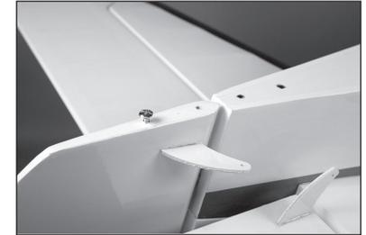
81. Remove the screws and apply 2-3 drops of thin CA into each hole.
