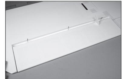
15. Fit the flap into position on the hinges.
