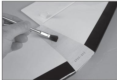
68. Use an epoxy brush to apply epoxy to the stabilizer mounting surface for the stabilizer. Position the stabilizer back on the fuselage and check its alignment. Use a paper towel and a small amount of isopropyl alcohol to remove any excess epoxy from the fuselage and stabilizer before the epoxy fully cures. Allow the epoxy to fully cure before proceeding.
