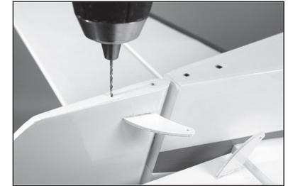
80. Thread an M2.5 x 10 sheet metal screw into each hole using a #2 Phillips screwdriver.
