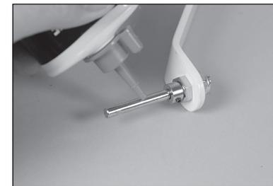
**107.** Fit the wheel to the axle, then install the remaining wheel collar on the axle. Make sure the setscrew is tightened on the flat area made on the axle.
