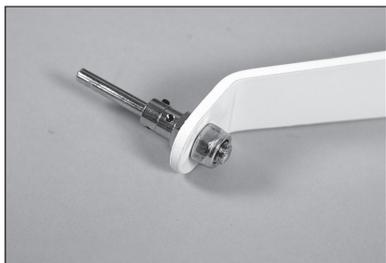
**105.** Loosen the setscrews in the wheel collars using a 1.5mm hex wrench. Remove the outer wheel collar. Slide the remaining wheel collar tight against the hex and tighten the setscrew.
