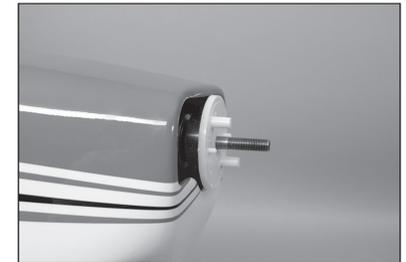
**164.** It may be necessary to trim the cowl to clear the muffler before the cowl can be properly aligned.
