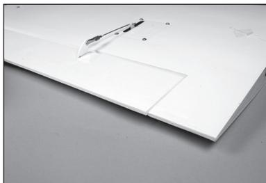
46. Move the control at the transmitter to the full flap position. Adjust the throw percentage of throw to achieve the 2<sup>11</sup>/<sub>32</sub> inches (60mm) full-flap throw.
