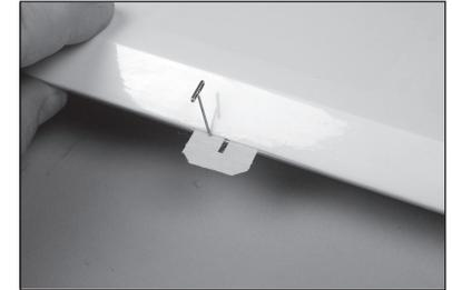
14. Fit the aileron into position on the hinges.
