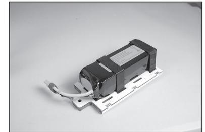
**129.** Slide the tray with the battery into the fuselage. The tray is then secured at the rear using a 1/4-20 nylon bolt.
