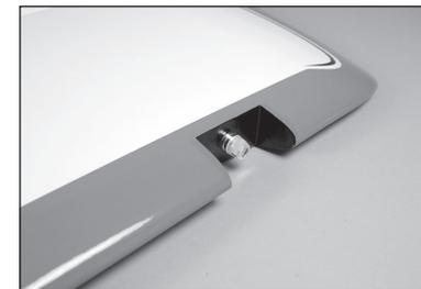
49. The landing light cover for the landing light is not symmetrical and will conform to the airfoil of the wing. Make sure it is oriented the correct direction when gluing it in place.
