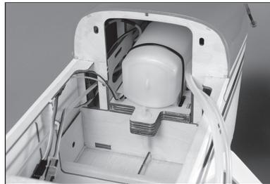
**160.** Install a fuel filler in the side of the fuselage and route the fuel fill line.
