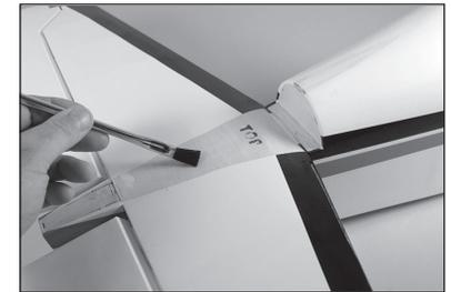
73. Use an epoxy brush to apply epoxy to the fin mounting surface.
