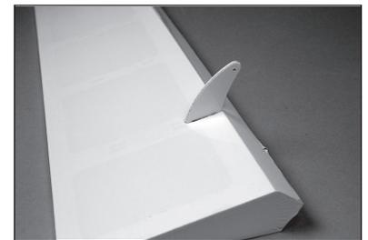
6. Use low-tack tape around the control horns to prevent epoxy from getting on the control surface.
