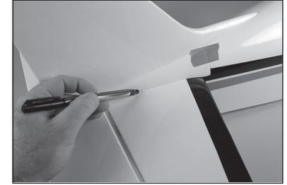
70. Trace the outline on the top of the fuselage using a felt-tipped pen.
