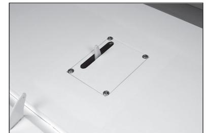
35. Locate the linkage for the ailerons. With the clevis removed, the linkage will measure  $3\frac{5}{32}$  inches (80mm).
