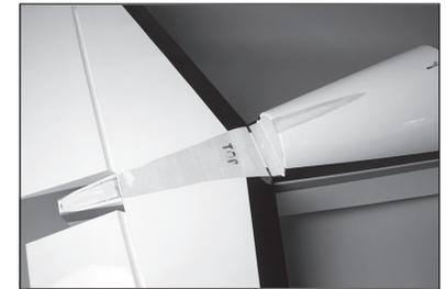
72. Mix 3/4 ounce (25ml) of 30-minute epoxy. Use an epoxy brush to apply epoxy to the exposed wood on the top of the stabilizer.
