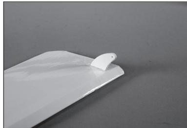
77. Hinge the rudder to the fin and fuselage using the techniques outlined previously in this manual.
