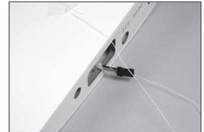
34. Secure the aileron servo cover using a #1 Phillips screwdriver and four M2.5 x 10 self-tapping screws.
