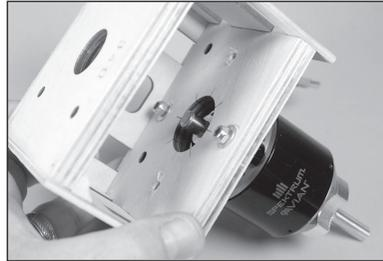
**114.** Position the motor box plate fully forward when using the recommended Spektrum Avian motor. The mount is adjustable for a variety of motors.
