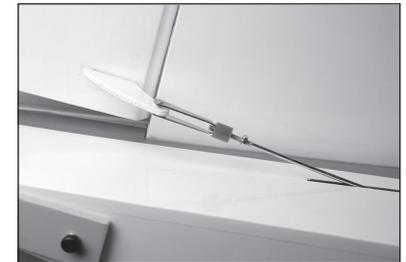
93. Slide the elevator pushrod connector on the pushrod from the servo. The pushrod will be in the center hole of the connector.
