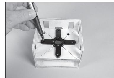
**111.** Remove the mount and drill the holes for the motor mounting screws using drill and 7/32-inch (5.5mm) drill bit.
