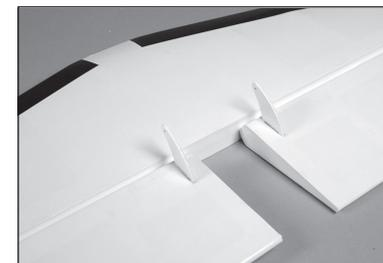
53. Use a small piece of low-tack tape to hold the elevators in alignment with the stabilizer for the next few steps.
