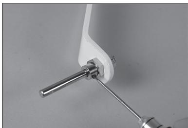
**106.** Apply a drop of light machine oil on the axle.
