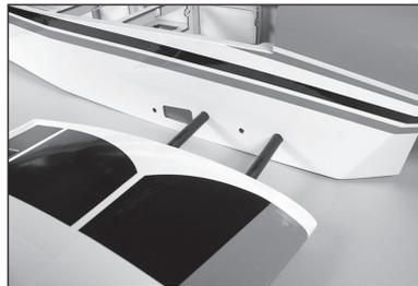
58. Secure the wing to the fuselage using two 1/4-20 x 1 nylon wing bolts.
