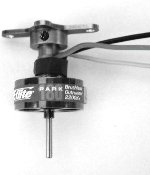
**NOTE:** Photo shows installation of x-mount onto the motor.
