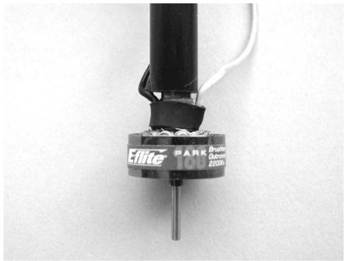
**NOTE:** Photo shows installation using a carbon fiber tube, with 7mm OD, 5mm ID (EFLM1963 available separately). This is an option for mounting the motor. You can cut down the carbon fiber tube to meet your specific needs and attach to your foam or wood airplane with glue.
