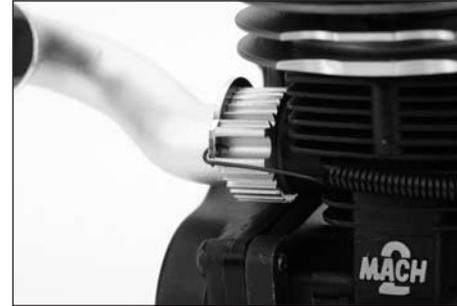
If your vehicle is supplied with a spring retention style manifold, use the supplied O-ring seal (DYN0719) along with the manifold gasket (DYNP5528) and retention spring.
