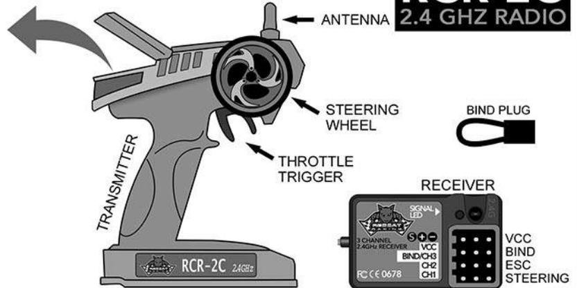
**Steering Reverse Switch:** Top left switch. Used to change steering orientation. If the car turns right when you steer left, flip this switch.
