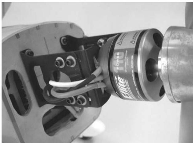
**NOTE:** Photo shows typical installation of motor directly to a separate electric motor mount such as the Hangar 9® EP Motor Mount with Hardware (HAN4245).
