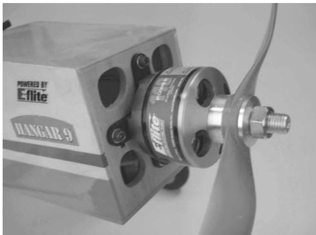
**NOTE:** Photo shows typical installation of motor and x-mount directly to the outside of the firewall. There are other options available including mounting the motor inside the fuselage or extending the motor further forward using aftermarket mount extensions when using cowls.
