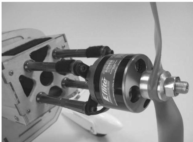
**NOTE:** Photo above shows installation using the Evolution™ Standoffs for Gas Engines (part numbers listed above). These standoffs work great for this application and are available in different sizes from 7mm up to 50mm in length. You can combine them to fit your exact needs. You will need to purchase socket head bolts to fit the customized standoffs lengths. Nylon motor standoffs (spacers) can also be used.
