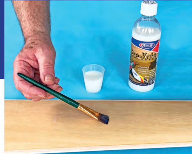
Apply an initial coat of Eze-Kote resin and allow it to dry.
