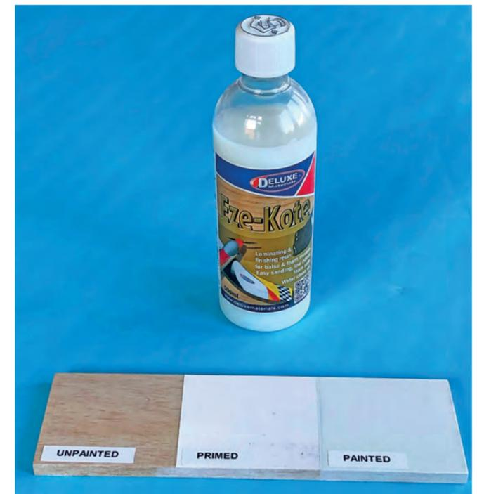
Having sanded the wing, Andy tested it using Halfords White Primer and his chosen paint, Halfords Spray Ford Diamond White. Eze-Kote has good compatibility with most white car primer paints. If you're in doubt always check by testing the primer and paint topcoat before committing it to the model.
