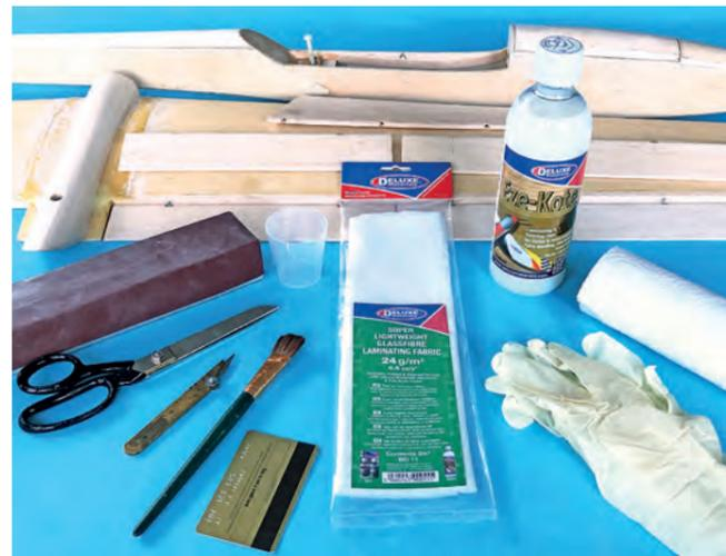
Eze-Kote (BD37) with the 0.6 oz super lightweight glass laminating fabric (BD11), gloves, brushes and scissors that you will need to undertake the Eze-Kote process.
