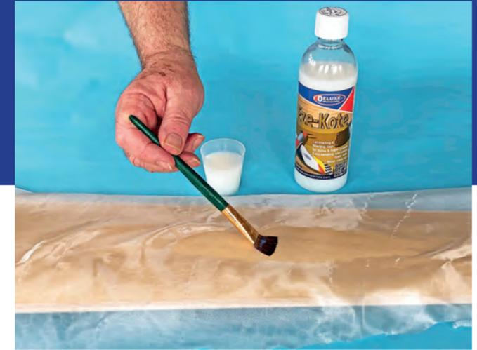
Eze-Kote is then brushed through the glass fibre fabric. Any unused Eze-Kote can be returned to its container.
