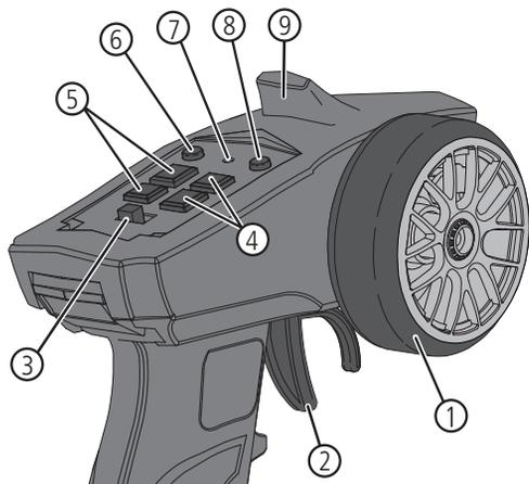
1. **Steering Wheel** Controls direction (left/right) of the model
