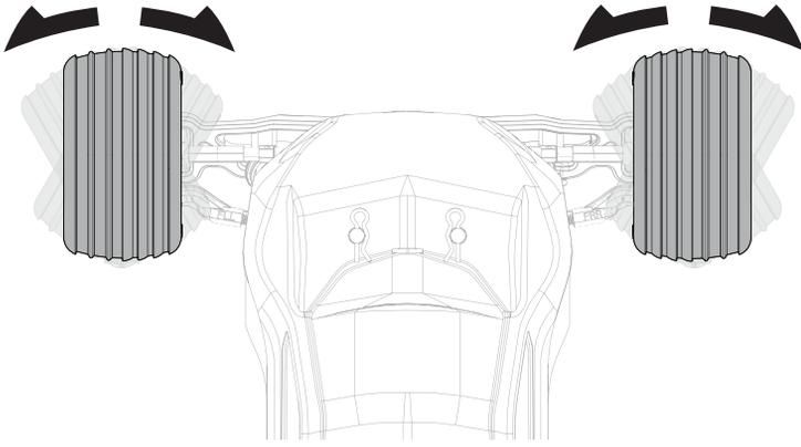
Perform a control test with the vehicle wheels off the ground. If the wheels rotate after the vehicle is powered ON, adjust the Throttle Trim until they stop. To make the wheels move forward, pull the trigger. To reverse them, wait for the wheels to stop, then push the trigger. When moving forward, the wheels should maintain a straight line without any steering wheel input. If not, adjust the Steering Trim, so the wheels maintain a straight line without having to turn the steering wheel.
