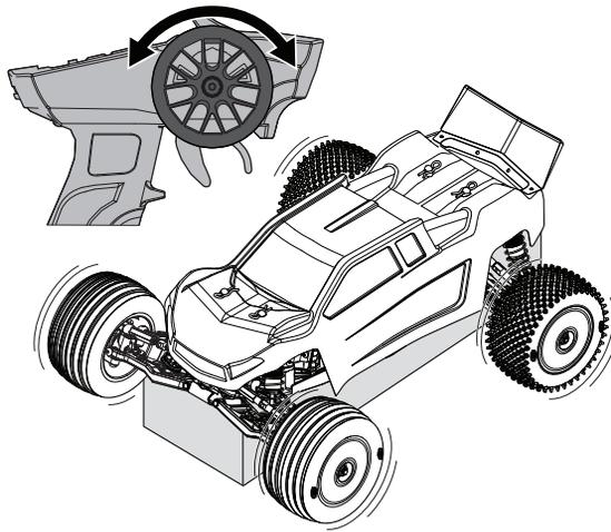
4. Start driving slowly, and, if the vehicle does not go straight, adjust the steering trim dial on the transmitter.
