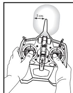
This illustration shows the approximate 5 cm RF exposure area and typical hand placement when operating your transmitter.
