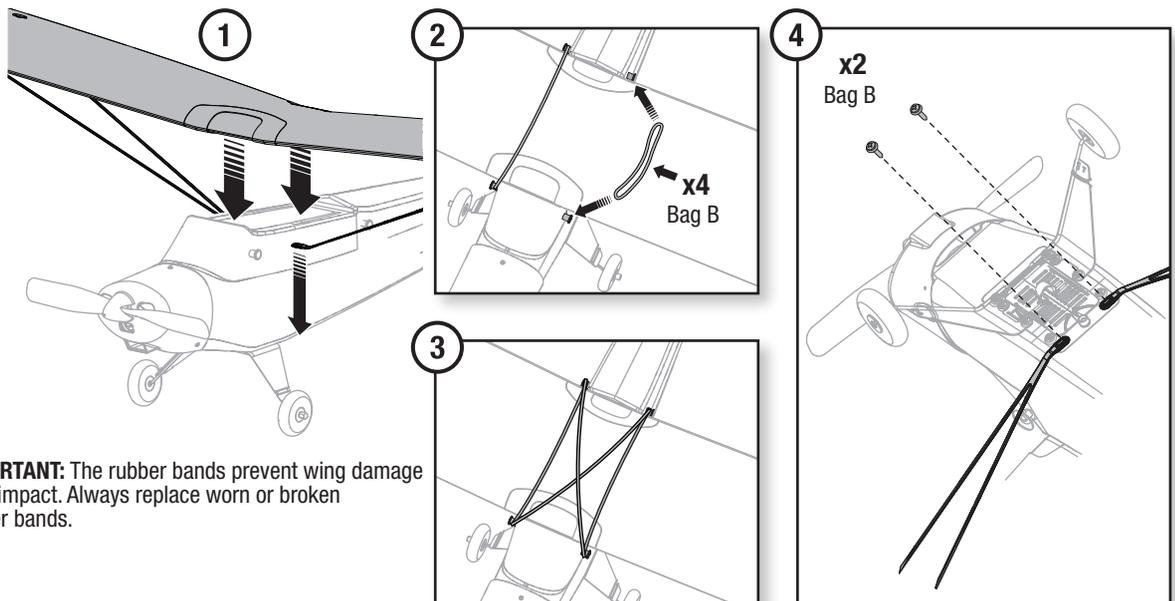
**IMPORTANT:** The rubber bands prevent wing damage from impact. Always replace worn or broken rubber bands.
