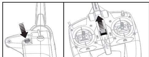
Press and hold the trainer button on the top of the transmitter while turning on the power switch.
