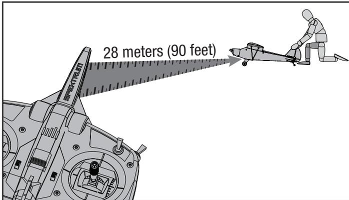
**CAUTION:** While holding the aircraft during the Range Test, always keep body parts and loose items away from the propeller. Failure to do so could cause personal injury.
