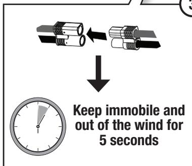
The aircraft can be held immobile for 5 seconds at any angle convenient for you to connect the battery.
