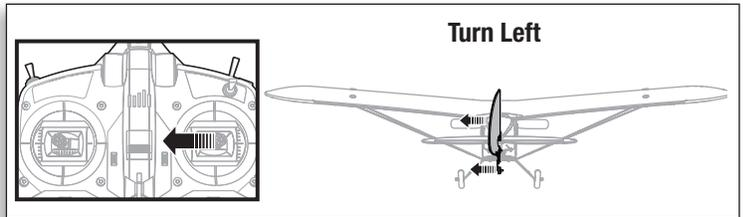
\*Mode 2 transmitter shown. For Mode 1, Elevator control is on the LEFT stick.
